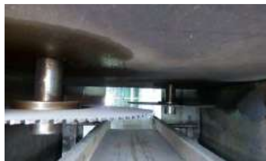
Adjustable rotating saw blades inside a fully housed and ventilated battery saw
