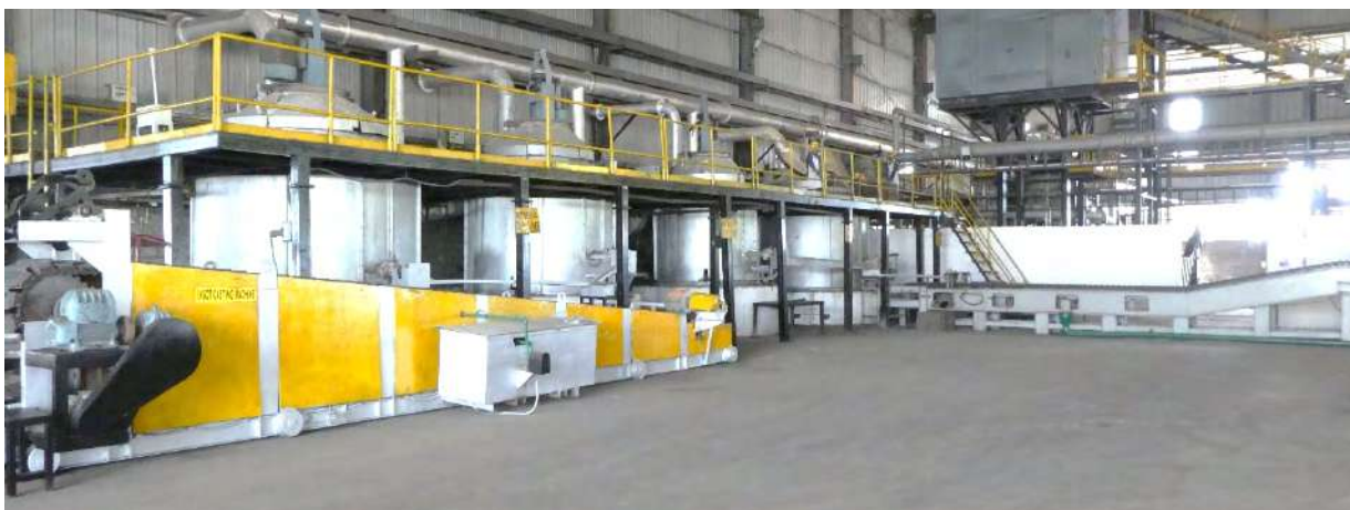
Elevated lead refining kettles with a gravity feed to casting machines adjacent to kettles 1 and 4
